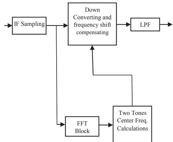
Fig.3. Calculation of Doppler frequency with FFT method in FSK modulation and its compensation
