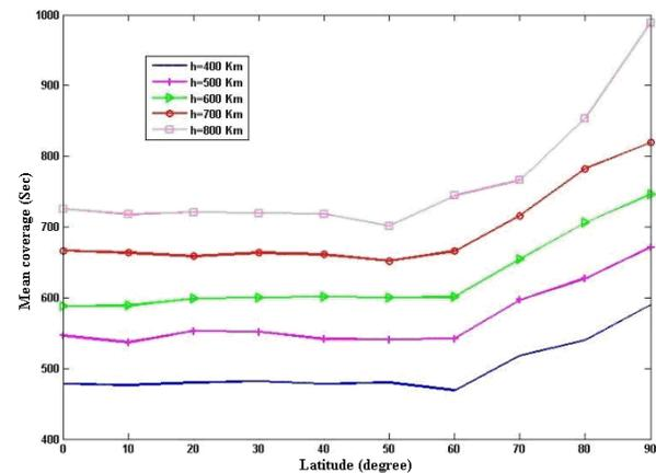
Fig. 4. Mean visibility time of one satellite pass in different latitudes and altitudes
