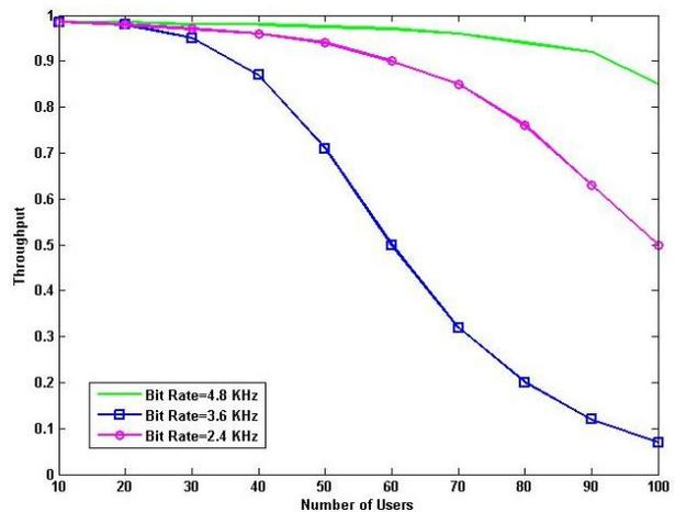
Fig.8. Simulation of SRMA throughput in terms of the number of users in random access time of 2 seconds with request signal length of 18 bytes and 4.5 kilobytes data
