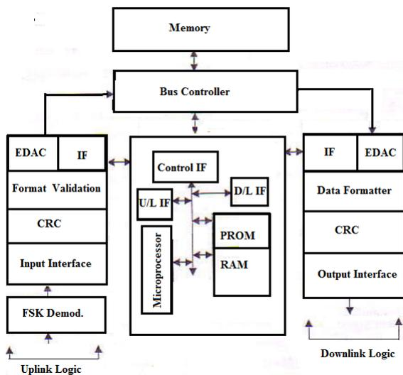
Fig. 12. Block diagram of uplink and downlink along with the microprocessor interface
