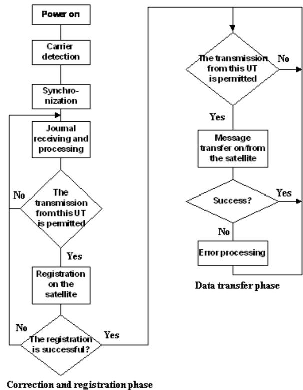
Fig. 13. Diagram of the user terminal functioning
