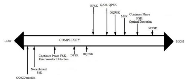
Fig.2. Complexity of different modulation methods
