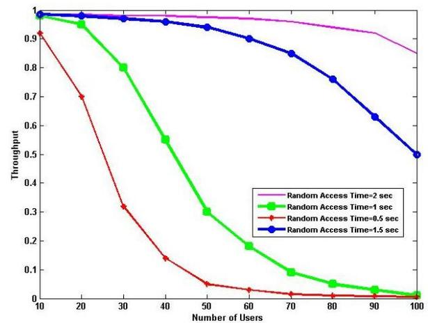
Fig.7. Simulation of SRMA throughput in terms of the number of users in bit rate of 4.8 kbps with request signal length of 18 bytes and 4.5 kilobytes data
