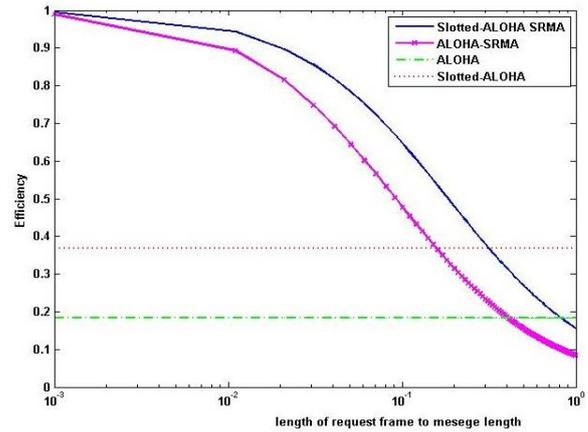
Fig.6. Efficiency of random access methods in terms of ratio of request frame length to the forwarded message packet
