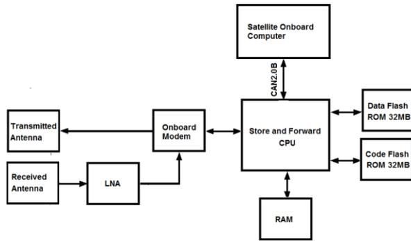
Fig. 11. Block diagram of developed S&F payload
