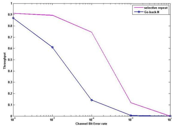
Fig.9. Efficiency of ARQ strategy in S&F payload in bit rate of 4.8 Kbps and altitude of 750 km
