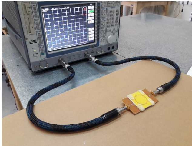
Fig. 9. Measurement setup for the fabricated circuit.
