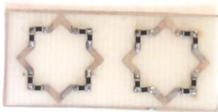
Fig. 7. The fabricated star-shape resistor loaded CA absorber
